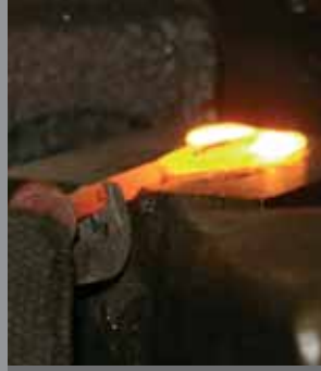
Drop forging a line pin blade.
