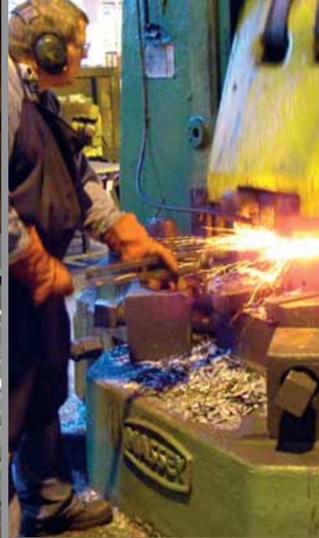
Drop forging Footprint brick bolsters. The carbon steel is heated to 1150°C before being placed over an impression of the tool to be forged. The "top" holds the top die which drops down to strike the steel over the bottom die.
