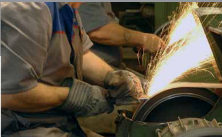
Hand grinding brick bolsters prior to heat treatment and painting.
